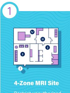
Restrict unauthorized entry to magnet through controlled access between zones.
